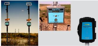
These meters use ultrasound to measure the speed of dirt, bubbles and other particles in the stream flow. Doppler meters transmit a sound wave into the flow. This sound wave is reflected by the particles in the water. The difference between the transmitted frequency and the received frequencies is proportional to the velocity of the flow.
