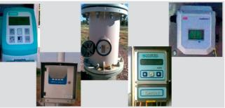
Electro-Magnetic flowmeters use Faraday's Law to determine the flow of water in a pipe. A magnetic field is generated around a flow tube. As the water passes through the magnetic field it causes a voltage signal which is sensed by electrodes located on the flow tube walls. When the water moves faster, more voltage is generated. The voltage generated is proportional to the flow rate.
