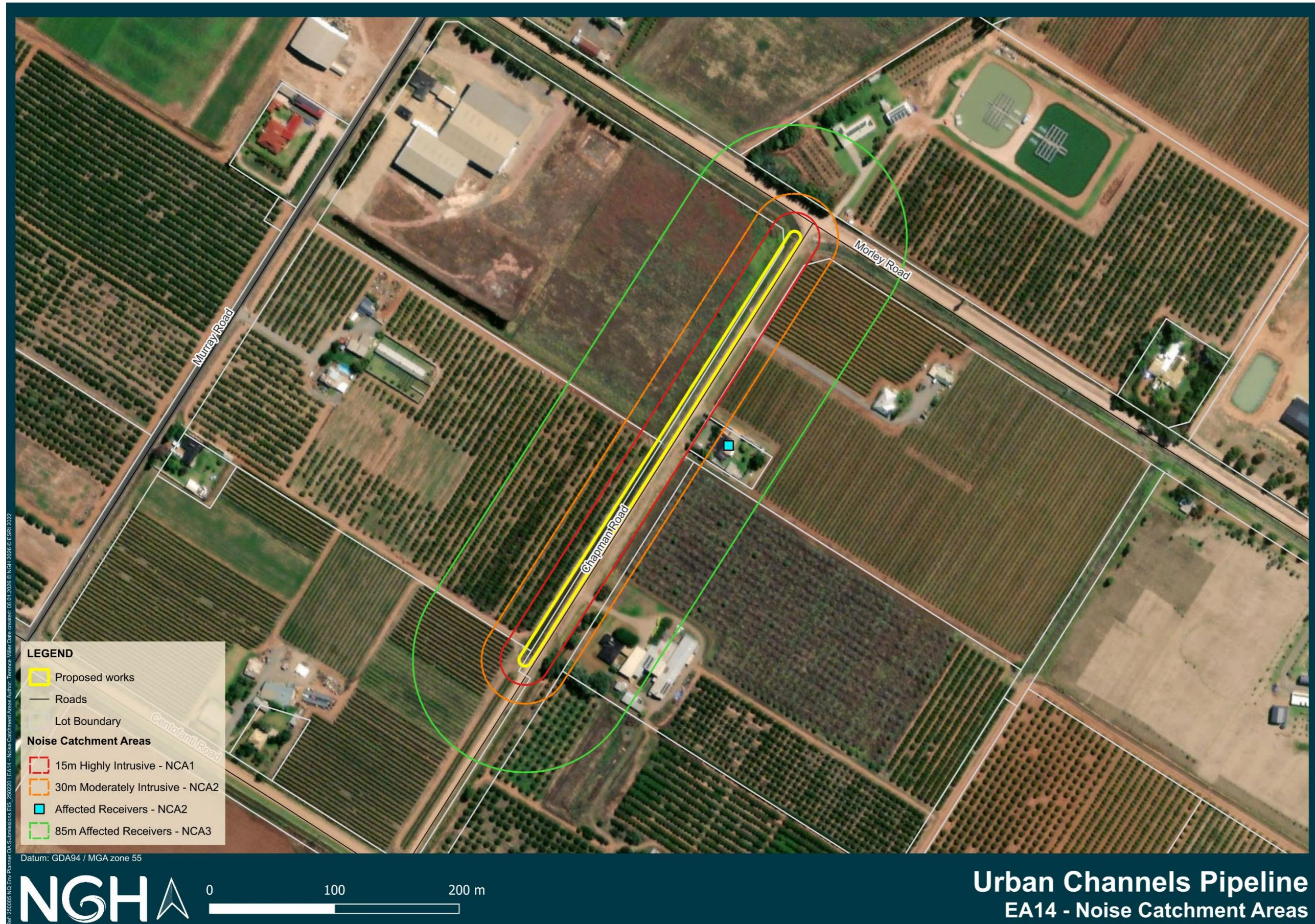
Figure 3-2 Noise catchment areas – standard construction works hours
