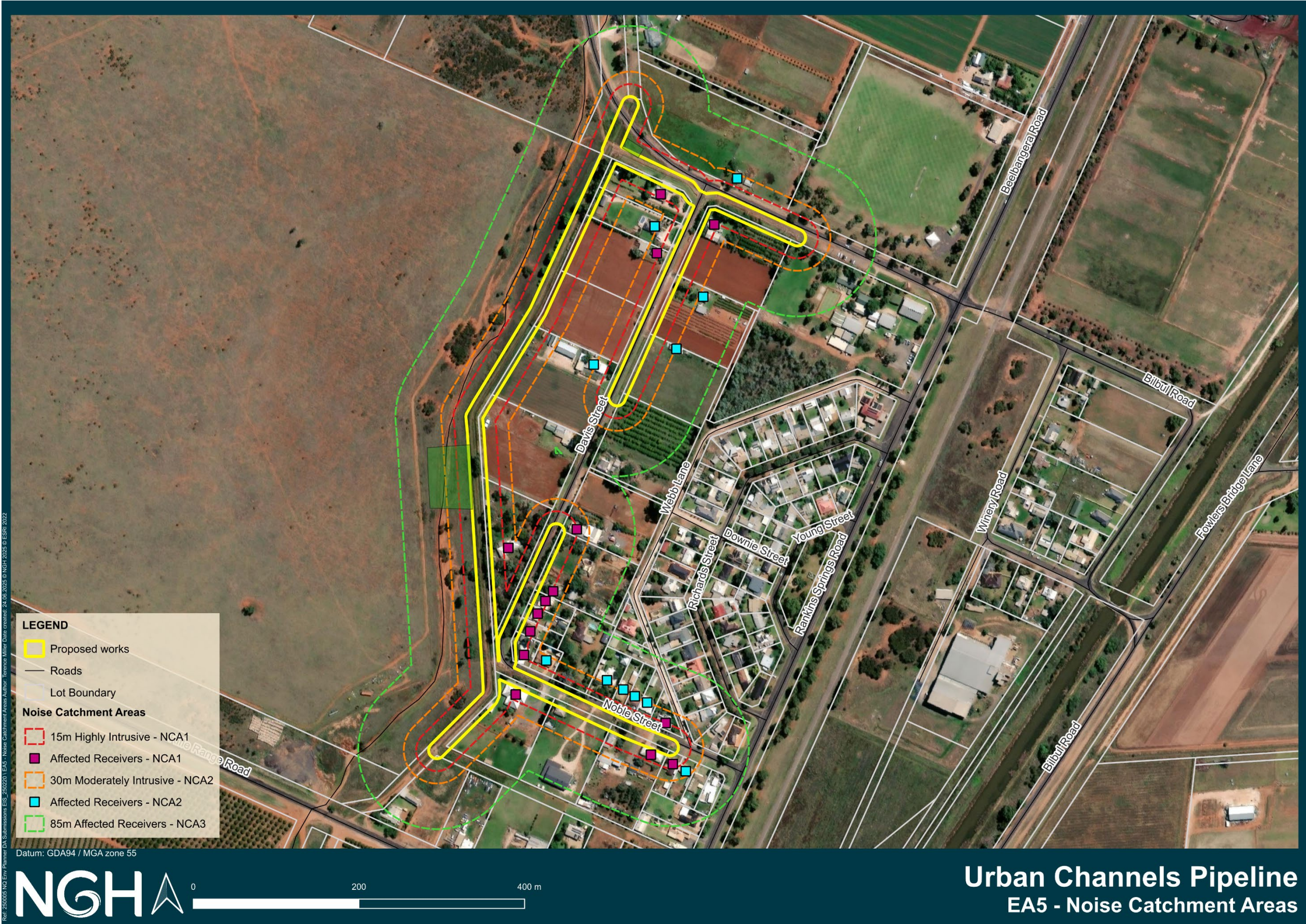
Figure 3-2 Noise catchment areas – standard construction work hours
