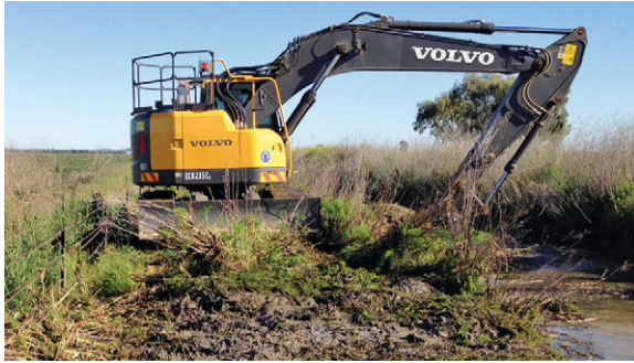
The zero-swing excavator allows us to work on narrow channel banks without damaging adjoining fencing.
