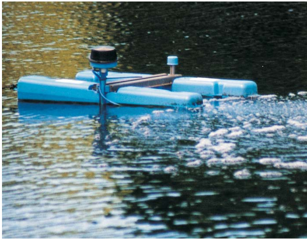
Figure 2. An aerator will help keep algae levels low
