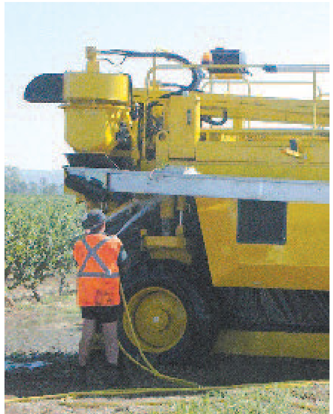
PHOTO: Harvesters must not be washed on channel banks. Use an on-farm basin area where the dirty water cannot return to the irrigation or drainage system.
